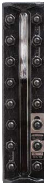
Reflex level gage showing about 60% oil
