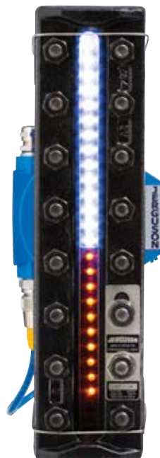
Transparent gage with illuminator showing 45% oil
